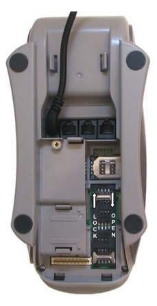
With **SIMcards** it is possible to access different services and to add new functions to the terminal. For example, a SIM card will be supplied by the bank to manage the Moneo electronic purse.
